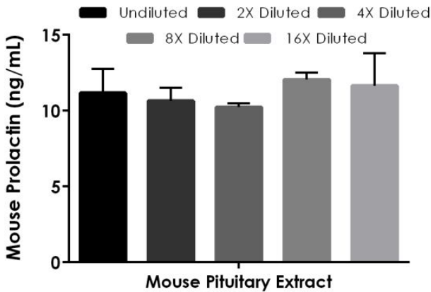
Figure 4. Interpolated concentrations of native Prolactin in mouse pituitary cell extract based on a 250 ng/mL extract load. The concentrations of Prolactin were measured in duplicate and interpolated from the Prolactin standard curve and corrected for sample dilution. The interpolated dilution factor corrected values are plotted (mean +/- SD, n=2). The mean Prolactin concentration was determined to be 20 ng/mL in mouse pituitary cell extract.
